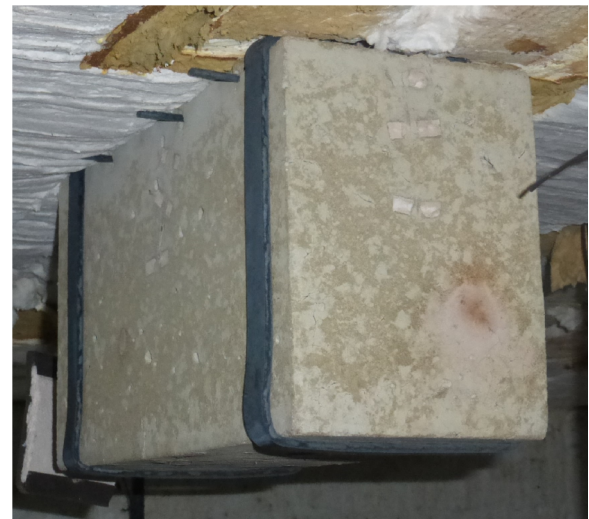
Fig. 25. Concrete block after fire exposure.
